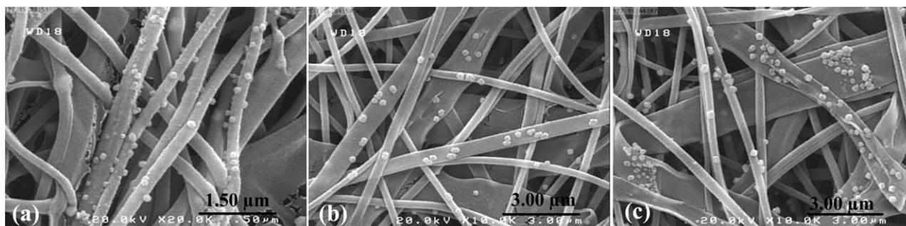
**Figure 3.** SEM micrographs of the CS/PEO/AgNO<sub>3</sub> nanofibrous mats with various salt concentrations, (a) 5.3 wt %, (b) 10.6 wt %, and (c) 21.2 wt % (Exp. A<sub>4</sub>–A<sub>6</sub>).
