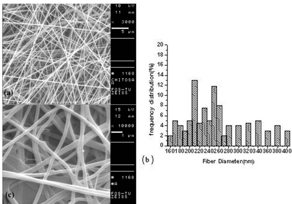
**Figure 1.** SEM image of the CS/PEO nanofibers from Exp. A<sub>1</sub> (a), its size distribution histogram of nanofibers (b), and SEM micrograph of the CS/PEO/AgNO<sub>3</sub> electrospun fibers of Exp. A<sub>2</sub> (c).
