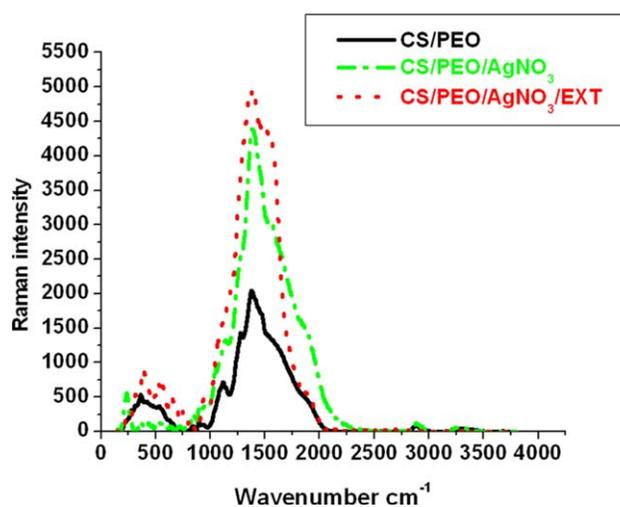
**Figure 5.** Raman spectra of CS/PEO (Exp. A<sub>1</sub>), CS/PEO/AgNO<sub>3</sub> (Exp. A<sub>2</sub>), and extract-incubated CS/PEO/AgNO<sub>3</sub> (Exp. A<sub>4</sub>) nanofibrous mats. [Color figure can be viewed in the online issue, which is available at [wileyonlinelibrary.com](http://wileyonlinelibrary.com).]
